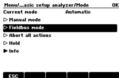
The *manual mode* of the analyzer is reserved for maintenance and repair work. This work must be done locally at the device, possibly by removing and replacing parts. Remotely requested activities cannot be allowed to interfere with this work and therefore are denied. Furthermore, it must not be possible to switch from manual mode to any other mode by remote command.
