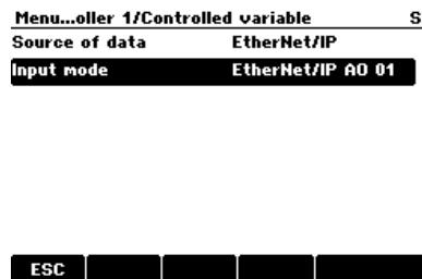
The value mapped to a device variable AO must be configured in the menu of the component using the device variable as input. A device variable AO is used to transmit an analog value to the measuring device instead of using a 4...20 mA current input of the measuring device.
