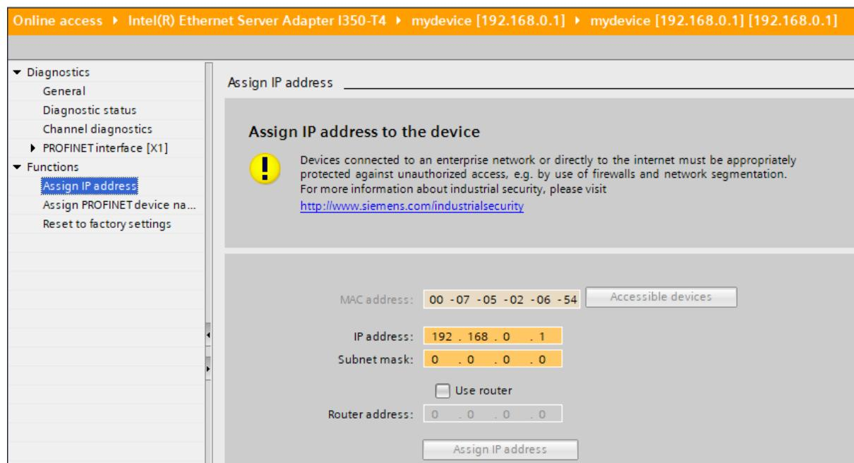
Simatic PRONETA *Reset Network Parameters* actually performs a RESET\_ALL\_STORED\_DATA.
