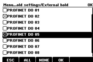
The value mapped to a device variable DO must be configured in the menu of the component using the device variable as input. A device variable DO is used to transmit an analog value to the measuring device instead of using a binary input of the measuring device.
