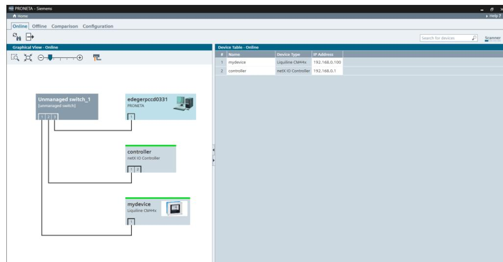
The device has now a valid IP address. If the device has a valid license for the integrated web server, you can access the web server directly from the context menu of SIMATIC PRONETA®.
