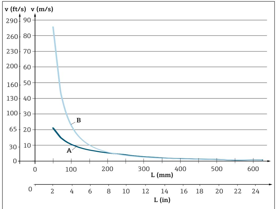
3 Permitted flow velocities, protection tube diameter 9 mm (0.35 in)
