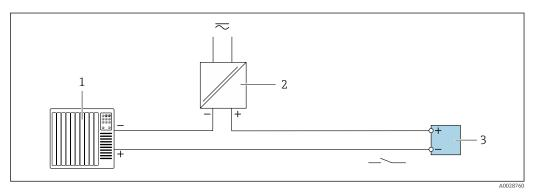
22 Connection example for relay output (passive)
