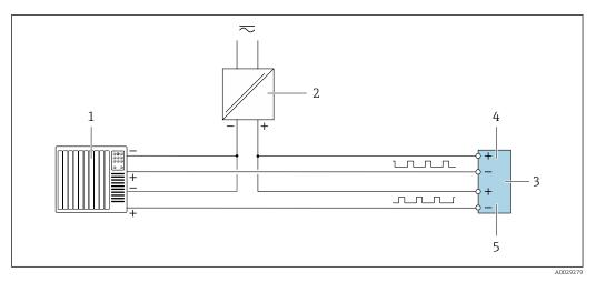
■ 26 Connection example for double pulse output (passive)
