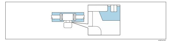
■ 8 Thermal insulation with not isolated extended neck
