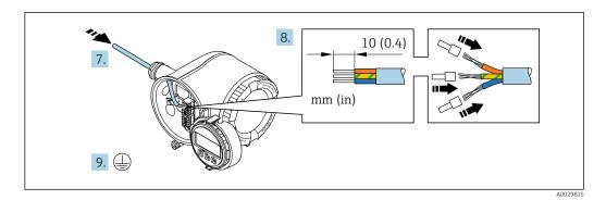
7. Push the cable through the cable entry. To ensure tight sealing, do not remove the sealing ring from the cable entry.
