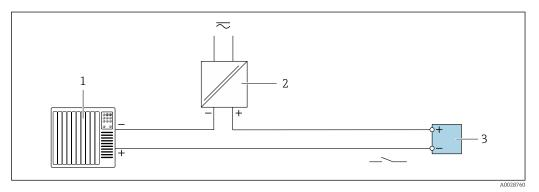
27 Connection example for relay output (passive)
