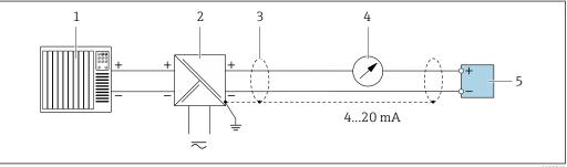
Connection example for 4 to 20 mA HART current output (passive)
