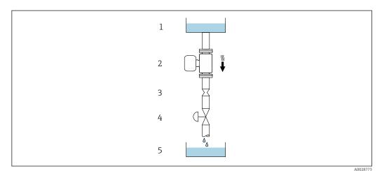
$\blacksquare$  6 Installation in a down pipe (e.g. for batching applications)
