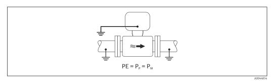
Connect the connection housing of the transmitter or sensor to ground potential by means of the ground terminal provided for this purpose.
