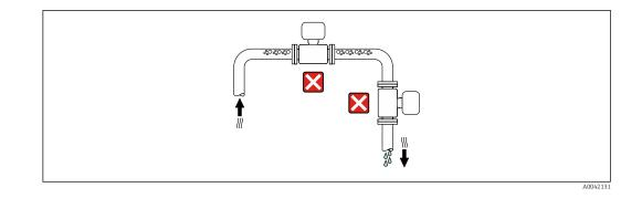
The device should ideally be installed in an ascending pipe.
