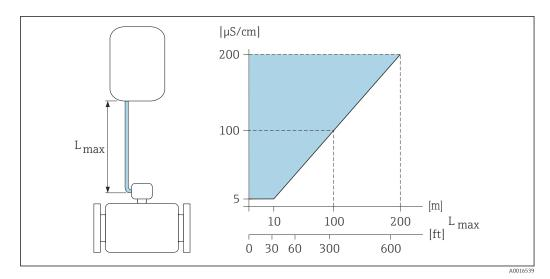
☑ 6 Permitted length of connecting cable Colored area = permitted range L<sub>max</sub>=length of connecting cable in [m] ([ft]) [µS/cm] = medium conductivity
