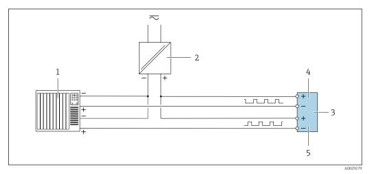
25 Connection example for double pulse output (passive)
