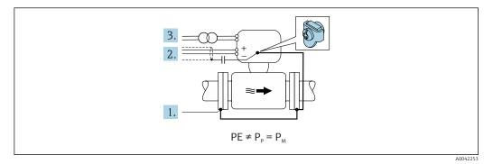
1. Connect the pipe flanges and transmitter via the ground cable.
