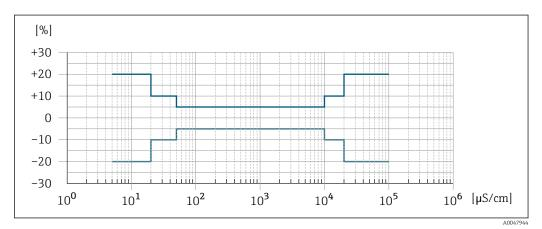
47 Measured error (optional: order code for "Calibrated conductivity measurement", option CW)
