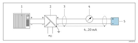
18 Connection example for 4 to 20 mA HART current output (passive)
