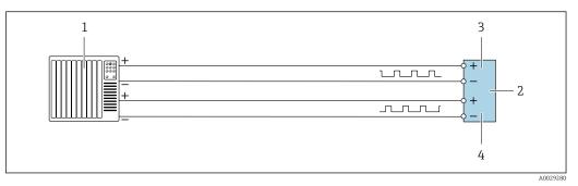
24 Connection example for double pulse output (active)
