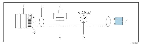
17 Connection example for 4 to 20 mA HART current output (active)
