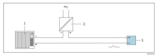
26 Connection example for relay output (passive)
