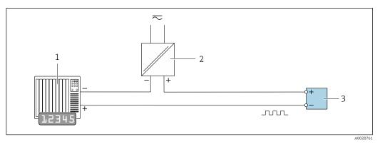
22 Connection example for pulse/frequency output (passive)
