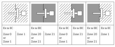
The device is designed for operation in explosive gas or explosive dust atmosphere as shown in the sketch above. In the event of potentially
