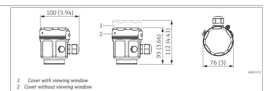
Engineering unit mm (in). Front view, left-hand side view, top view Thread depth of cable gland 10 mm (0.39 in) max.
