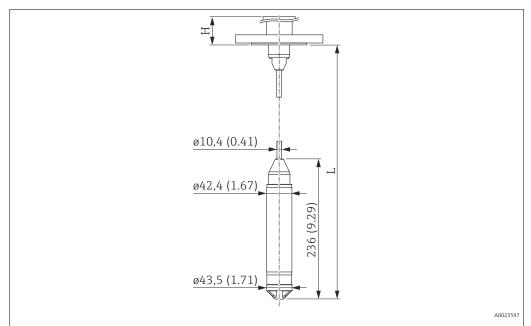
For dimensions of process connections Probe length L=500 to  $300\,000$  mm (20 to  $11\,810$  in) - see Product Configurator, order code for "Probe" connection"
