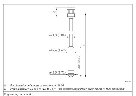
Process connection incl. measuring cell
