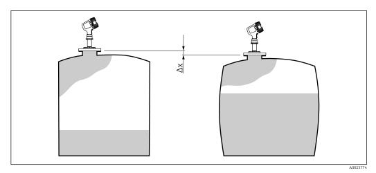
■ 21 Movement ∆x of the Gauge Reference Height due to the bulging of the tank shell caused by hydrostatic pressure
