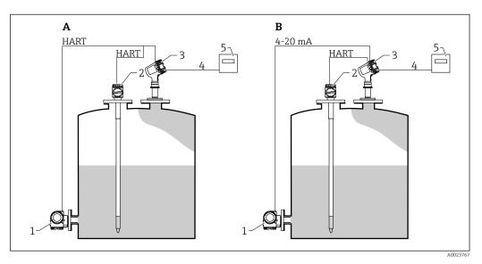
■ 3 Integration of tank sensors with Micropilot (Example)
