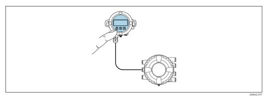
■ 18 Operation via remote display and operating module DKX001
