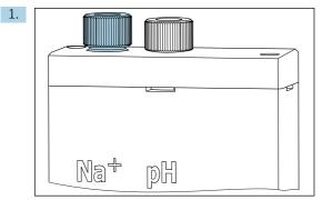
Loosen the screw connection on the measuring unit.
