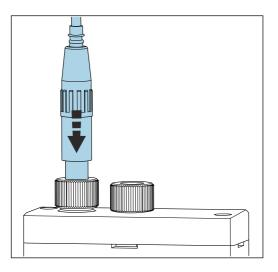
Carefully insert the electrode as far as it will go into the left-hand chamber (sodium) or right-hand chamber (pH).
