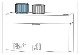
Loosen the screw connection on the measuring unit.
