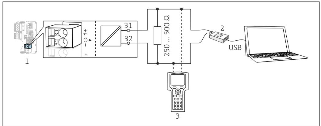
12 Mediante modem HART
