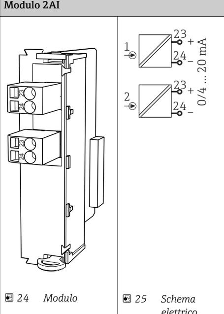
The diagram shows the physical layout of the 2AI module on the left and its electrical schematic on the right. The schematic shows two channels, labeled 1 and 2. Each channel has two terminals, labeled 23 and 24. The schematic also includes symbols for current input, such as triangles with arrows and circles with arrows. The current range is specified as 0/4 ... 20 mA.
