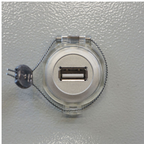
29 USB port sealed with sealing wire
