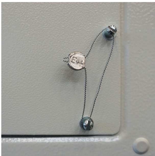
27 Screws sealed with sealing wire
