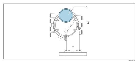
$\blacksquare$  31 Pressure gauge and gas purging nozzle
