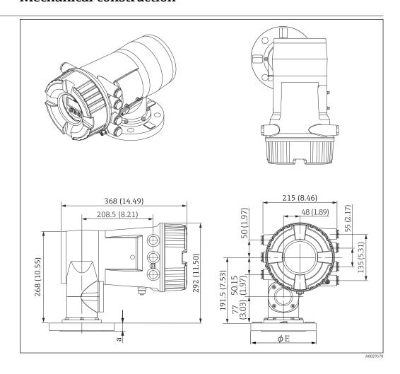
Flanges according to ASME B16.5, Pressure rating 150 lbs 1)
