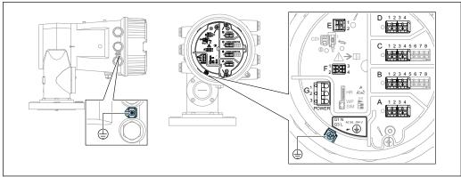
lacksquare 11 Terminal compartment (typical example) and ground terminals
