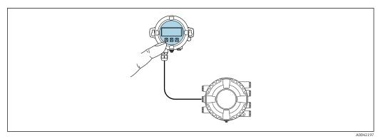
■ 21 Operation via remote display and operating module DKX001
