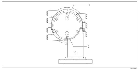
$\blacksquare$  29 Holes for cleaning nozzle and gas purging nozzle
