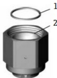
Fig 71. Centering gasket on bonnet seal surface
