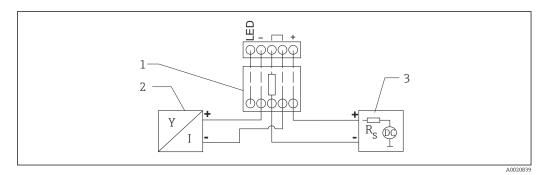
■ 4 Block diagram; device connection, RIA15 without light, HART communication resistor
