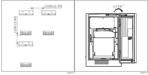
I3 Minimum spacing required for mounting. If Maximum opening angle Engineering unit mm (in).
