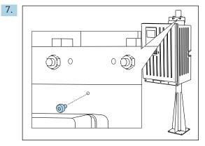
Fix the upper wall holder unit in place with the screw provided.
