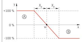
Red: overlap between the curves of the two 1-sided controllers.
