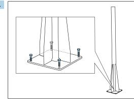
Erect the post and mount it securely on the foundation using 4 fixing screws (to be provided by the customer  $^{1)}$ ).
