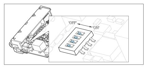
🖻 44 DIP switch for internal termination
