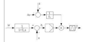
Strictly speaking, feedforward control involves an open-loop control system, since its effect is not measured directly. That means that the feed flow is directed exclusively forward. Hence the designation "feedforward control".
