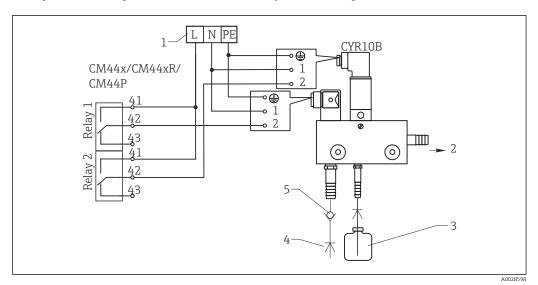
■ 39 Connecting the CYR10 injector cleaning unit
