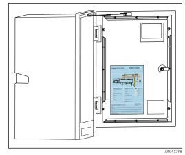
The diagrams below reflect the status at the time of issue of this documentation. The hose connection diagram that applies for your device version is provided on the inside of the door of the analyzer.
