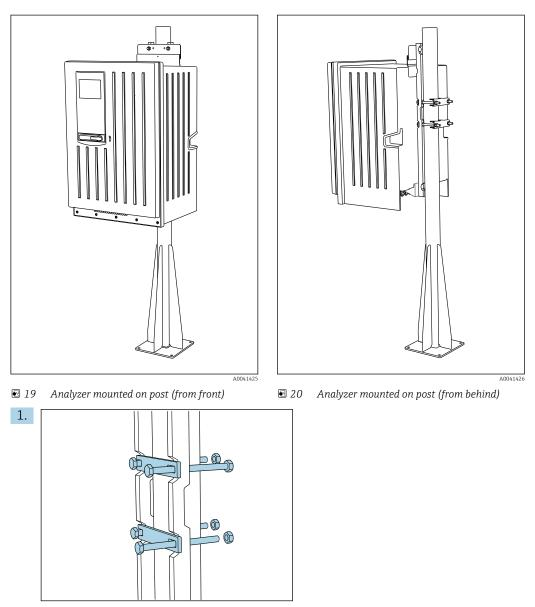
Fit the clamp of the post retainer on the retaining rods and post using the nuts.
