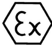
Figure 1. ATEX label for use in hazardous areas
