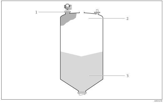
Flange: Reference point of measurement 20 mA, 100% 1
