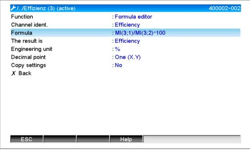
The counter values of mathematics channel 1 and 2 must be used to calculate the efficiency. "Efficiency" must be selected for the "The result is" parameter. With this setting, the counter values of the signal analysis are automatically used for efficiency calculation and you receive 4 efficiency values (e.g. 15 min, day, month, year) to display and save.
