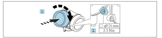
1. Screw down the cover of the electronics compartment.
