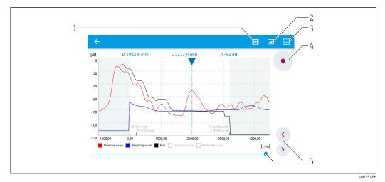
🖻 29 Envelope curve display (sample) in SmartBlue for Android
