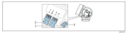
■ 15 Terminal assignment, 4-wire: 4 to 20 mAHART (90 to 253 V<sub>AC</sub>)
