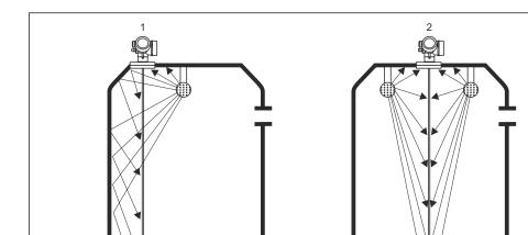
Tanks with spray ball for probe cleaning
