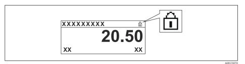
If hardware write protection is disabled, no option is displayed in the **Locking status** parameter. On the local display, the 🖻 symbol disappears from in front of the parameters in the header of the operational display and in the navigation view.
