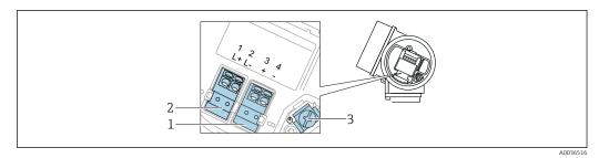
$\blacksquare$  13 Terminal assignment, 4-wire: 4 to 20 mA HART (10.4 to 48 V<sub>DC</sub>)
