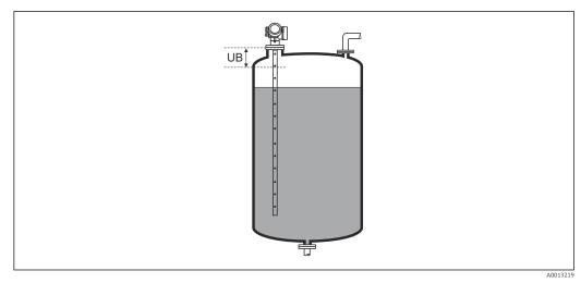
■ 43 Blocking distance (UB) for liquid measurements
