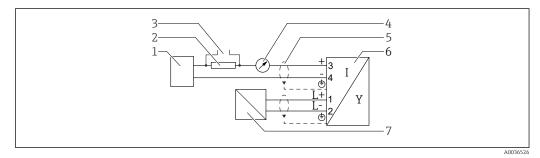
■ 14 Block diagram, 4-wire: 4 to 20 mA HART (10.4 to 48 V<sub>DC</sub>)
