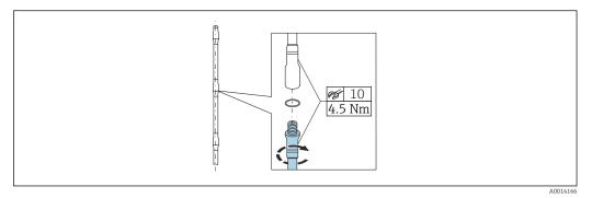
The use of separable rod probes ( $\emptyset$  8 mm) is advisable in confined mounting conditions (limited distance to the ceiling).
