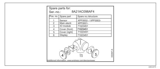
35 Example for spare part nameplate in the connection compartment cover
