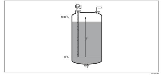
Full calibration (F) for level measurements in liquids 🛃 40
