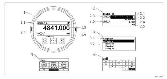
**2**7 Display format on the display and operating module
