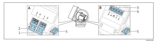
■ 11 Terminal assignment, 2-wire: 4 to 20 mA HART, 4 to 20 mA
