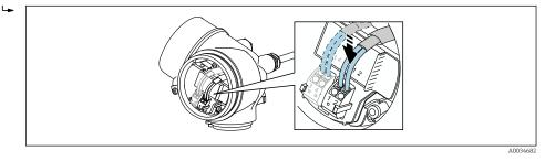
6. If using shielded cables: Connect the cable shield to the ground terminal.
