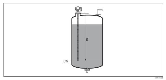
☑ 39 Empty calibration (E) for level measurements in liquids
