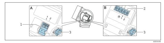
Image: Terminal assignment, 2-wire: 4 to 20 mA HART
