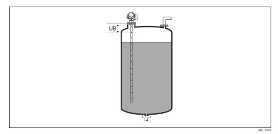
Blocking distance (UB) for liquid measurements
