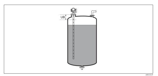
■ 39 Blocking distance (UB) for liquid measurements
