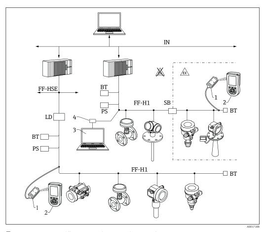
$\blacksquare$  17 FOUNDATION Fieldbus system architecture with associated components
