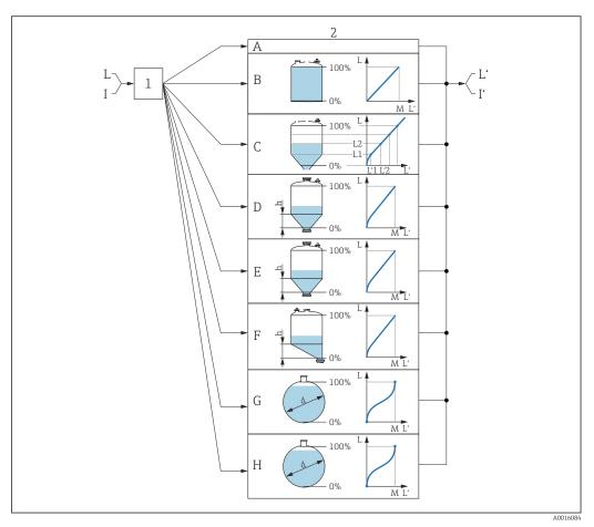
**■** 37 Linearization: Conversion of the level and, if applicable, interface into a volume or a weight; the conversion depends on the vessel shape
