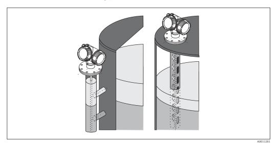
■ 4 Mounting position of Levelflex FMP55
