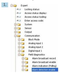
In the FieldCare navigation window, navigate to **Expert**  $\rightarrow$  **Communication**  $\rightarrow$  **Field** diagnostics  $\rightarrow$  Alarm detection enable.
