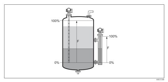
■ 34 Full calibration (F) for interface measurements
