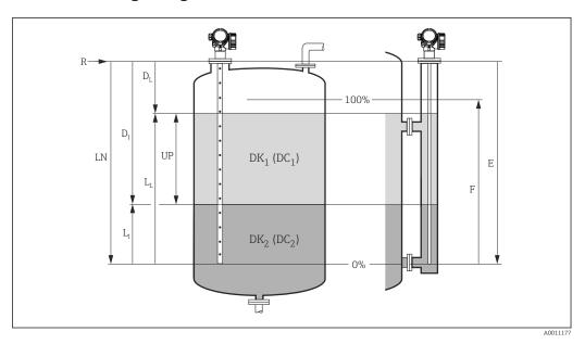
■ 22 Configuration parameters for interface measurement
