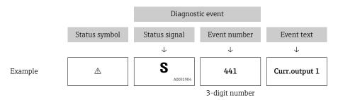
If two or more diagnostic events occur simultaneously, only the diagnostic message with the highest priority is shown. Additional queued diagnostic messages can be shown in the **Diagnostic list** submenu.
