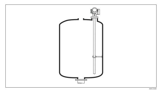
Coax probes can be secured (fixed) at any point in the ground tube.
