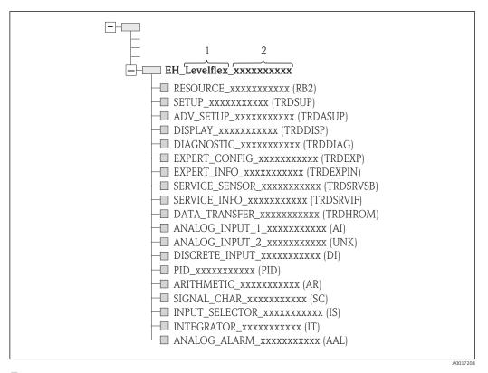
$\blacksquare~19~$  Typical display in a configuration program after the connection has been established
