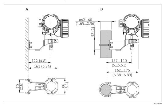
■ 6 Mounting the electronics housing with the mounting bracket. Unit of measurement mm (in)
