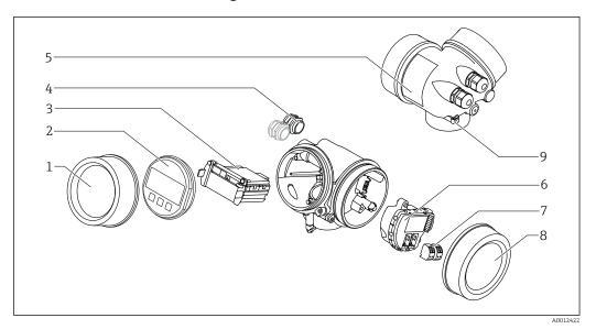
**₽** 2 Design of the electronics housing
