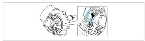
6. If using shielded cables: Connect the cable shield to the ground terminal.
