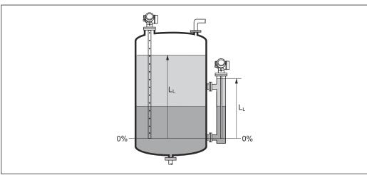
■ 35 Level in case of interface measurements
