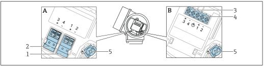
■ 9 Terminal assignment PROFIBUS PA / FOUNDATION Fieldbus
