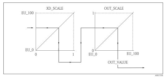
■ 24 Scaling the measured value in the AI Block
