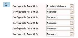
Select one of these bits (here for example: **Configurable Area Bit 1**) and select the **In safety distance** option from the corresponding selection list. Press Enter to confirm the option selected.
