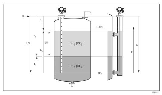
25 Configuration parameters for interface measurement
