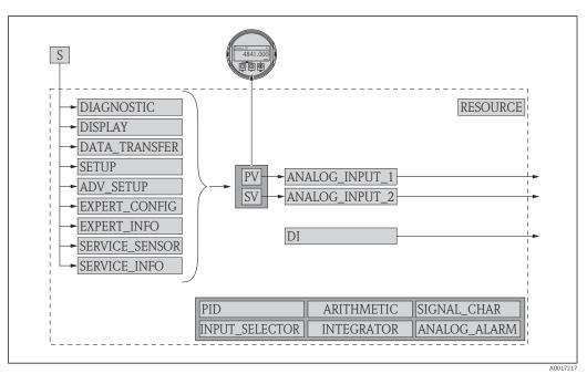
■ 20 Block configuration when device is delivered
