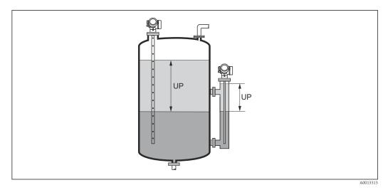
UP Interface thickness (= thickness of upper medium)
