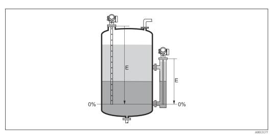
■ 33 Empty calibration (E) for interface measurements
