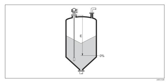
■ 40 Empty calibration (E) for level measurements in bulk solids.
