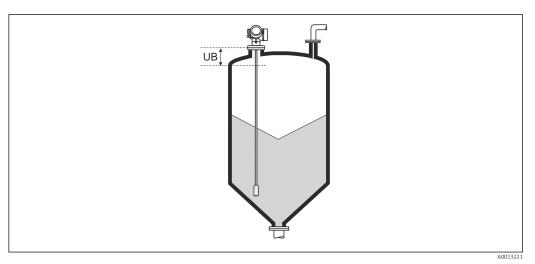
■ 47 Blocking distance (UB) for bulk solid measurements
