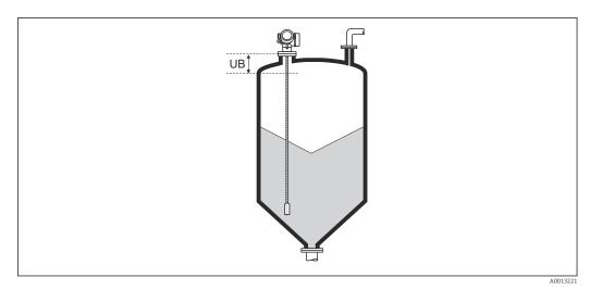
■ 44 Blocking distance (UB) for bulk solid measurements
