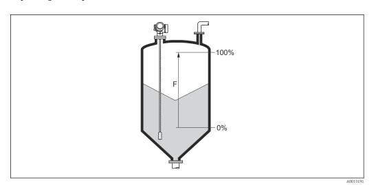
$\blacksquare$  41 Full calibration (F) for level measurements in bulk solids
