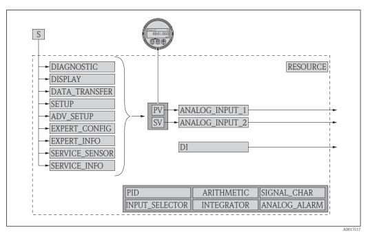
■ 26 Block configuration when device is delivered
