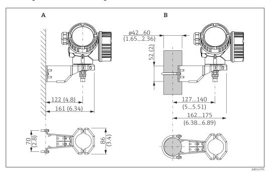
$\blacksquare~12~$  Mounting the electronics housing with the mounting bracket. Unit of measurement mm (in)
