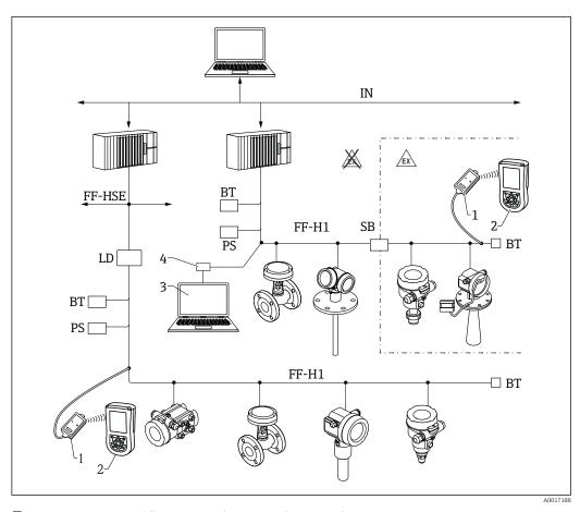
$\blacksquare$  23 FOUNDATION Fieldbus system architecture with associated components
