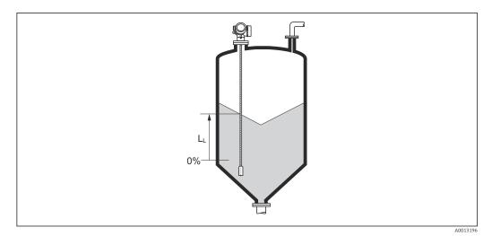
■ 42 Level in case of bulk solid measurements
