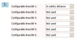
Select one of these bits (here for example: **Configurable Area Bit 1**) and select the **In safety distance** option from the corresponding selection list. Press Enter to confirm the option selected.
