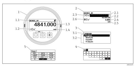
■ 24 Display format on the display and operating module
