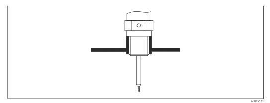
₩ 9 Mounting with threaded connection; flush with the vessel ceiling
