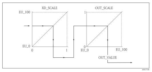
■ 30 Scaling the measured value in the AI Block
