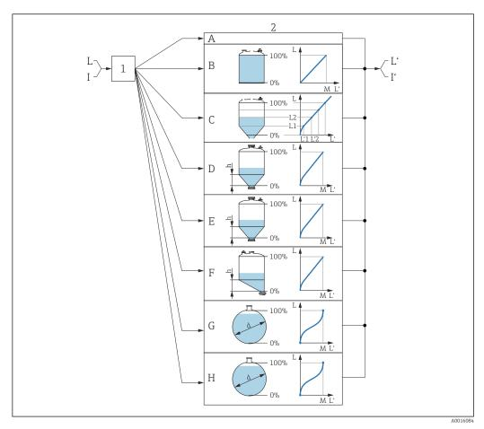
45 Linearization: Conversion of the level and, if applicable, interface into a volume or a weight; the conversion depends on the vessel shape
