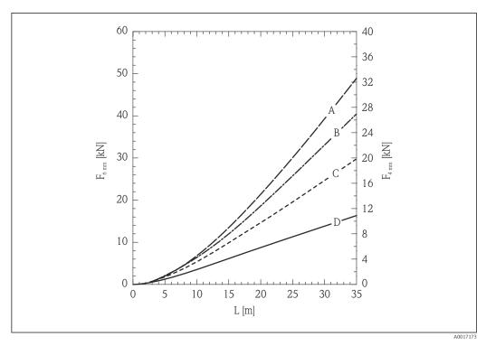
8 Cement in metal silo with smooth walls; tensile load as a function of level L for rope diameters
