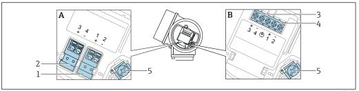
■ 15 Terminal assignment PROFIBUS PA / FOUNDATION Fieldbus
