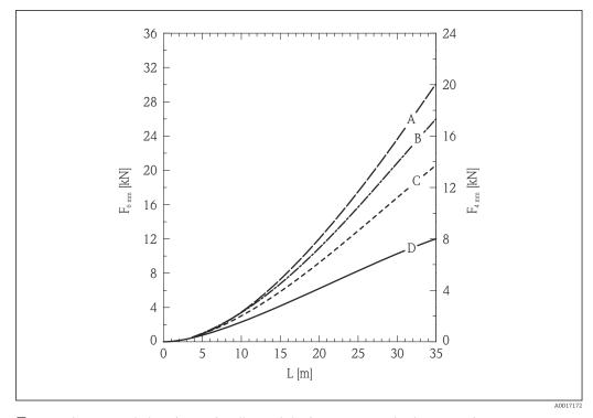
$\blacksquare$  7 Wheat in metal silo with smooth walls; tensile load as a function of level L for rope diameters 6 mm (0.24 in) and 4 mm (0.16 in)
