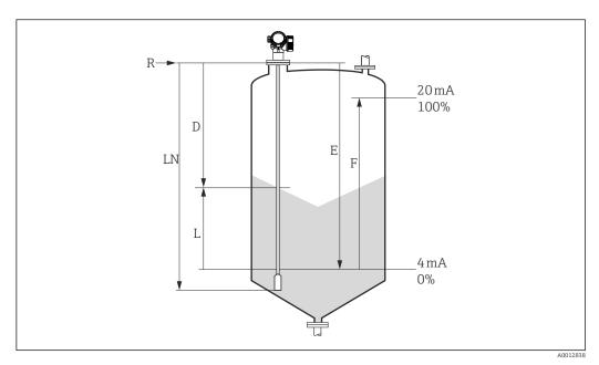
$\blacksquare$  31 Configuration parameters for level measurement in bulk solids
