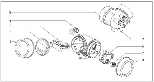
**₽** 2 Design of the electronics housing
