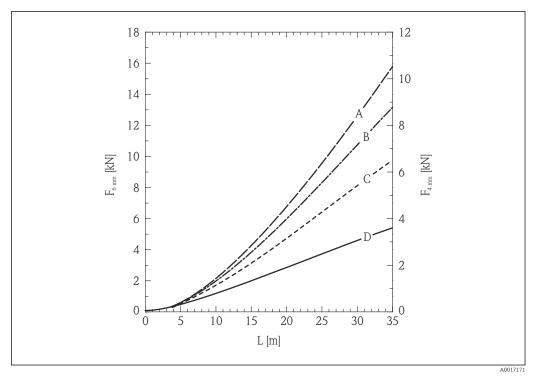
Polyethylene pellets in metal silo with smooth walls; tensile load as a function of level L for rope diameters 6 mm (0.24 in) and 4 mm (0.16 in)
