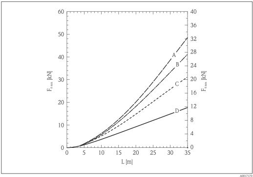
**₽** 5 Silica sand in metal silo with smooth walls; tensile load as a function of level L for rope diameters 6 mm (0.24 in) and 4 mm (0.16 in)
