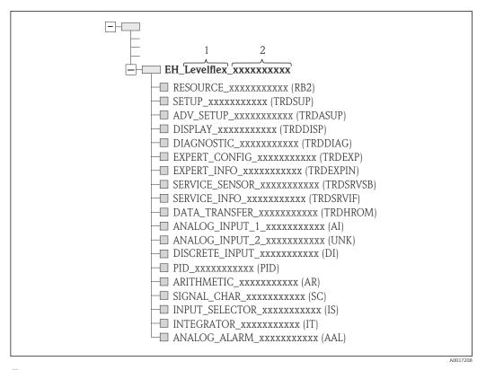
■ 25 Typical display in a configuration program after the connection has been established
