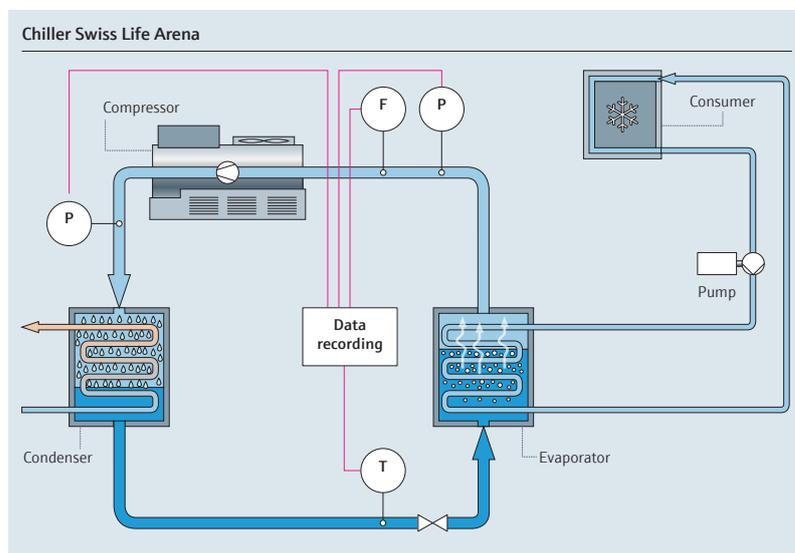
Measuring technology used: Proline Promass F 300 (top photo, measuring point F in graphic), Cerabar PMP51B (photo at bottom left, measuring points P in graphic), Resistance thermometer TR15 (photo at bottom right, measuring point T in graphic) as well as Memograph M RSG45 (photo at bottom center, "Data recording" in graphic)
