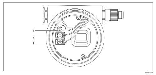
I Connection terminals and ground terminal in the connection compartment
