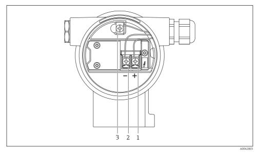
2 Connection terminals and ground terminal in the connection compartment
