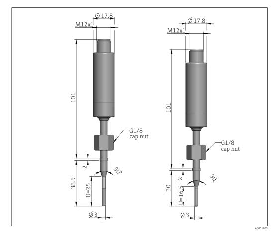
12 *Thermometer with metal sealing system 30°, G1/8 cap-nut (dimensions in mm)*
