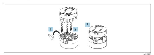
■ 17 Attach the display to the transmitter
