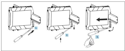
$\blacksquare$  8 Dismantling the DIN rail transmitter
