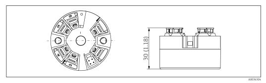
21 Version with push-in terminals. Dimensions are identical to the version with screw terminals, apart from housing height.
