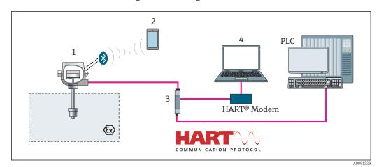
$\blacksquare$  15 Operation options for the transmitter via HART® communication
