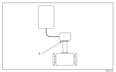
Position of reference point for temperature measurement
