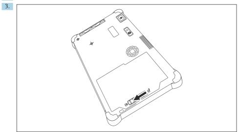
Slide the battery lock into the "Locked" position. The battery is inserted.
