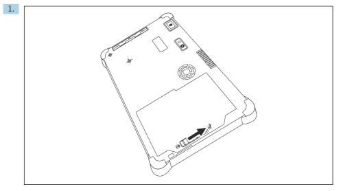
Slide the battery lock into the "Unlocked" position.
