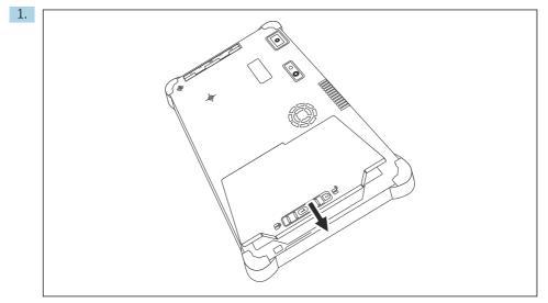
Insert the battery in the battery compartment.
