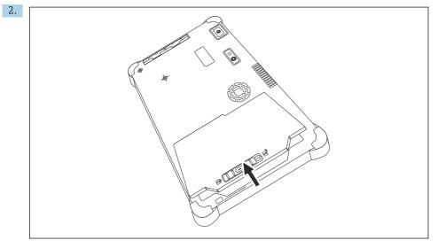
Open the battery compartment and remove the battery.
