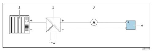
External verification taking the example of a passive current output
