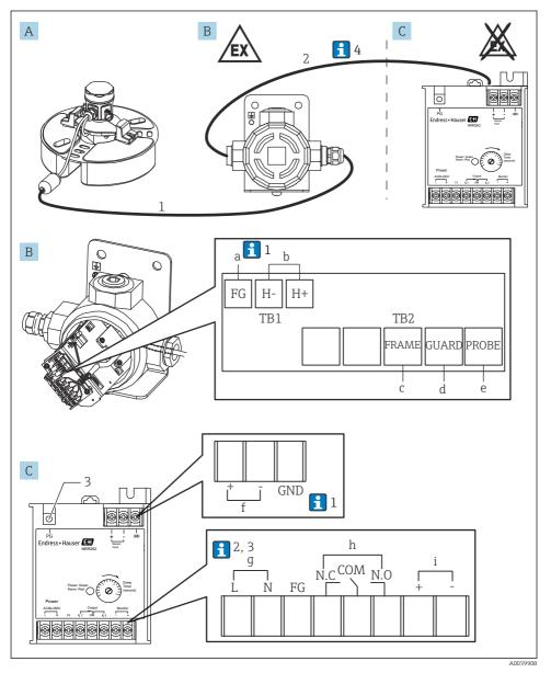
■ 12 Wiring of Ex [ia] Converter NRR262-4/A/B/C
