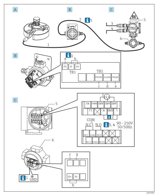
13 Wiring of Ex d [ia] Converter NRR261-5
