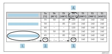
I Procedure for determining the temperature class and surface temperature
