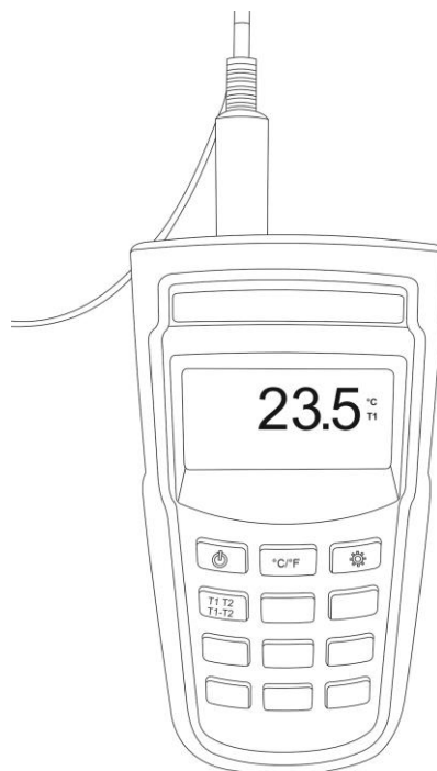
Figure 12. Thermometer inserted into the temperature measurement port
