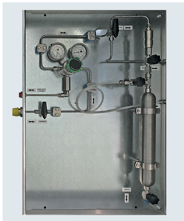
Special portable equipment for on-site fluid sampling from the diagnostic chamber
