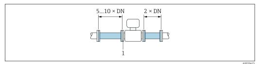
$lap{1}{1}$  Recommended inlet and outlet runs when using a flow conditioner
