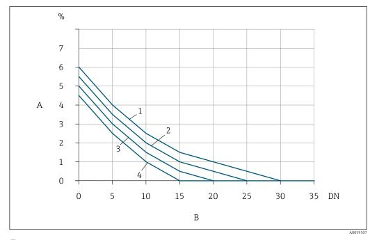
The additional measured error to be expected without flow conditioners depending on the disturbance type and inlet run
