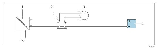
■ 27 Connection example for 4 to 20 mA current input
