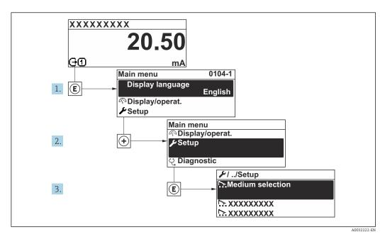
$\blacksquare$  37 Navigation to "Setup" menu using the example of the local display
