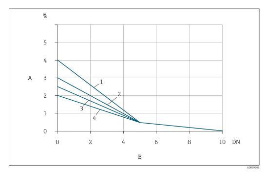
The additional measured error to be expected with flow conditioners depending on the disturbance type and inlet run
