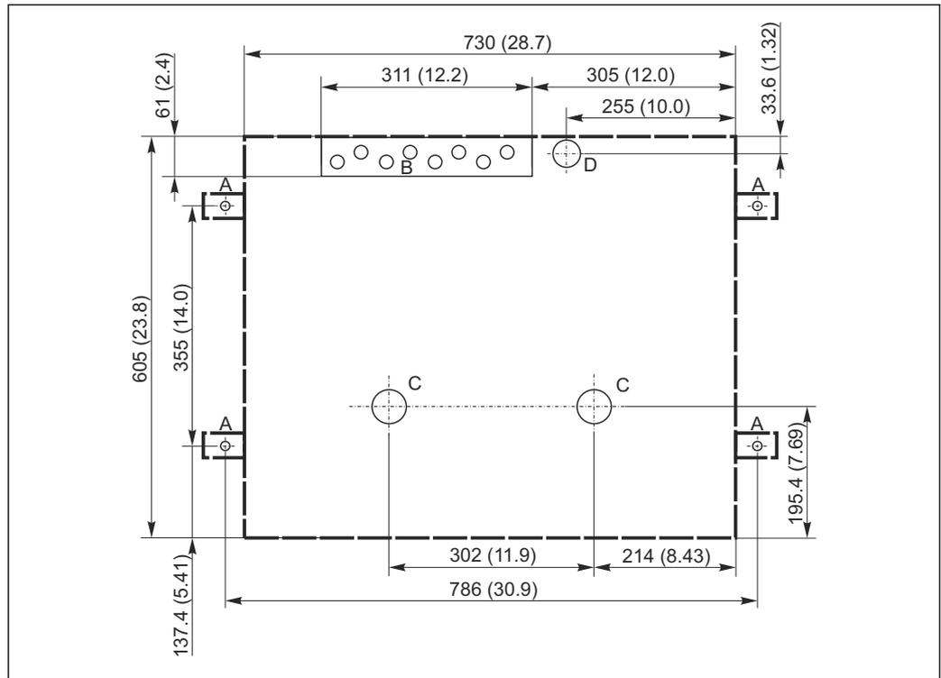
5 Foundation plan. Unit of measurement mm (in)
