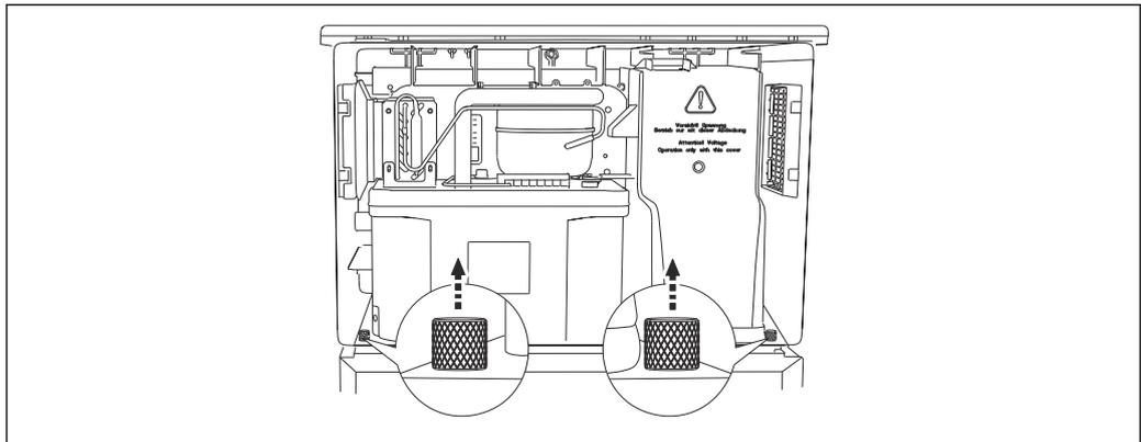
1. Remove the bolt on the rear of the dosing compartment.
