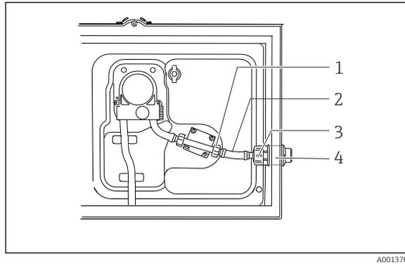
9 Connecting the suction line from the side (as-delivered state)
