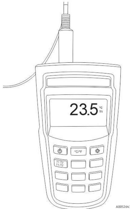
Figure 15. Thermometer inserted into the temperature measurement port
