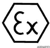
Figure 6. ATEX label for use in hazardous areas
