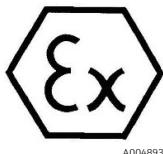
Figure 3. ATEX label for use in hazardous areas
