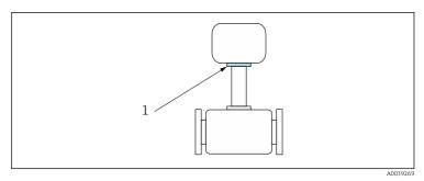
■ 1 Position of reference point for temperature measurement
