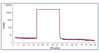
The chart above depicts the output of a Endress+Hauser TDLAS gas analyzer to a large "slug" of moisture in a natural gas stream. Note the rapid response at the beginning of the event ("wet-up"), and at the end ("dry-down").
