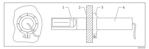
■ 8 Rod sensor mounted, rear view
