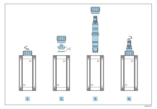
1 Dummy plug and O-ring
