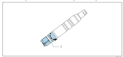
$\blacksquare$  8 Screw on membrane cap: keep pressure relief valve clear.
