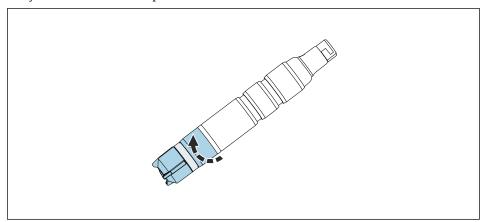
► Carefully remove membrane cap.
