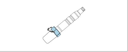
► Carefully remove protection cap from sensor.
