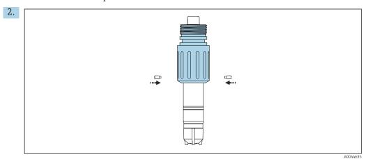
Fix the adapter with the 2 stud screws supplied and an Allen screw (2 mm (0.08 in)).
