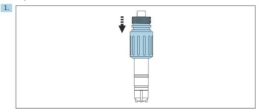
Starting from the sensor head, slide the adapter for Flexdip CYA112 onto the sensor as far as the end stop.
