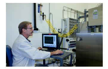
Standard analyzer testing includes a 30-minute zero, onehour nominal, and one-hour high range test. Extended repeatability testing for all analytes (except  $O_2$ ) are available. For  $H_2O$  measurements greater than 50 ppm, factory review is required.
