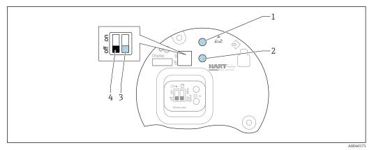
■ 24 Operating keys and DIP switch on FEL60H electronic insert
