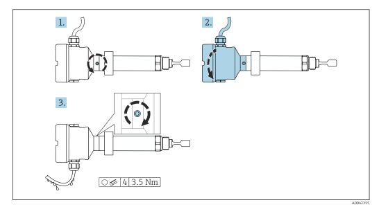
■ 14 Housing with external locking screw and drip loop
