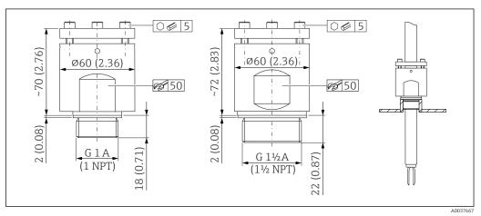
■ 30 High pressure sliding sleeves. Unit of measurement mm (in)
