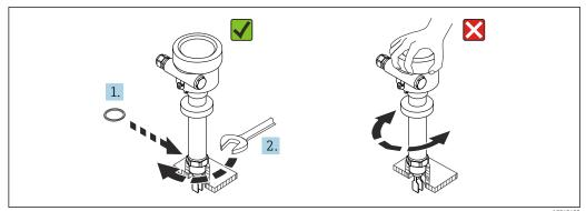
**■** 13 Screwing in the device
