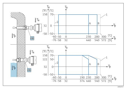
$\mathbb{Z}$  32 Permitted ambient temperature  $T_n$  at the housing as a function of the process temperature  $T_n$  in the vessel
