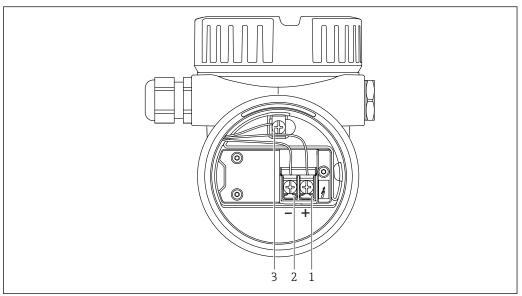
Connection terminals and ground terminal in the connection compartment
