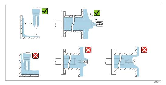
$\blacksquare$  8 Installation examples for a highly viscous process medium
