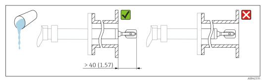
$\blacksquare$  7 Installation example for a highly viscous liquid. Unit of measurement mm (in)
