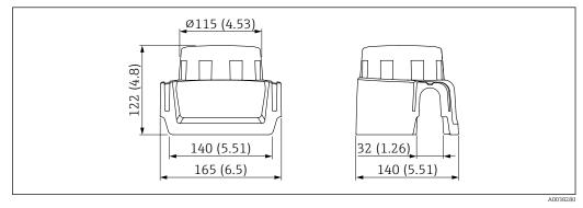
■ 28 Protective cover for single compartment housing, aluminum or 316L. Unit of measurement mm (in)
