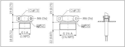
Sliding sleeves for unpressurized operation  $p_e = 0$  bar (0 psi). Unit of measurement mm (in)
