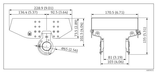
■ 27 Protective cover for aluminum dual compartment housing. Unit of measurement mm (in)
