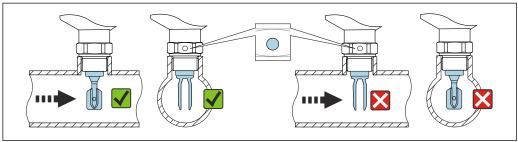
Installation in pipes (take fork position and marking into consideration)
