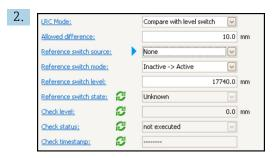
Go to the **LRC Mode** parameter and select the **Compare with level switch** option.
