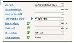
Go to the **LRC Mode** parameter and select the **Compare with level device** option.
