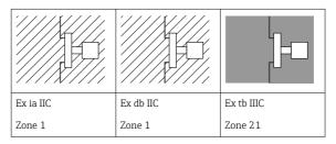
The device is designed for operation in explosive gas or explosive dust atmosphere as shown in the sketch above. In the event of potentially explosive gas-air and dust-air mixtures occurring simultaneously: Suitability requires further assessment.
