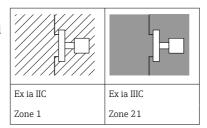
The device is designed for operation in explosive gas or explosive dust atmosphere as shown in the sketch above. In the event of potentially explosive gas-air and dust-air mixtures occurring simultaneously: Suitability requires further assessment.
