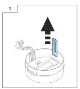
Only when using with FEL68: Activating the battery
