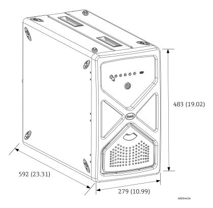
Figure 6. Raman Rxn2 analyzer. Dimensions: mm (in)
