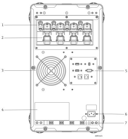
Figure 4. Rear panel of Raman Rxn2 four-channel analyzer
