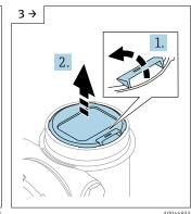
If fitted: release the screw of the cover lock for the display cover using the Allen key.
