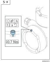
▶ If fitted: release the screw of the cover lock for the connection compartment cover using the Allen key.
