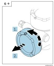
Unscrew the connection compartment cover, check the cover seal. Screw this cover onto the electronics compartment instead of the display cover. If fitted: tighten
