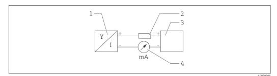
■ 4 Block diagram of HART connection
