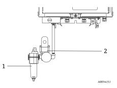
Figure 4. Purge regulator and filter assembly
