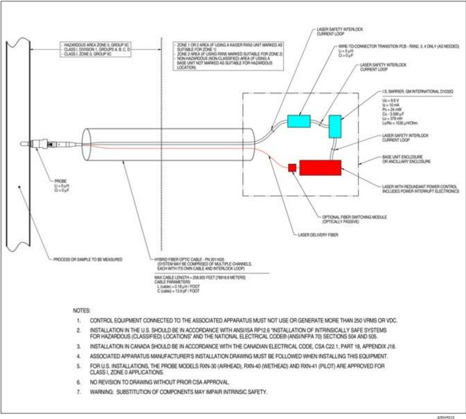
Figure 10. Control drawing for probe I.S. circuit (4002396 X6)
