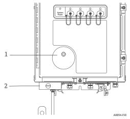
Figure 3. Purge indicator and valve system
